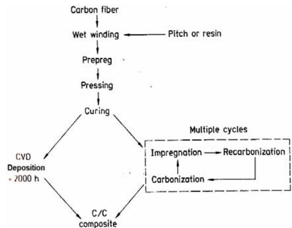
Figure 1 Carbon – carbon manufacturing process
