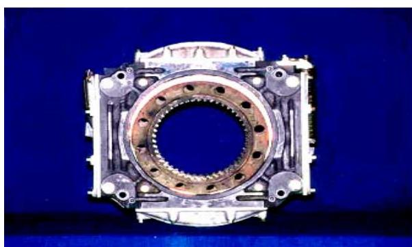
Figure 3 Double disc dry type hydraulic actuated 32 brake shoes/assembly
