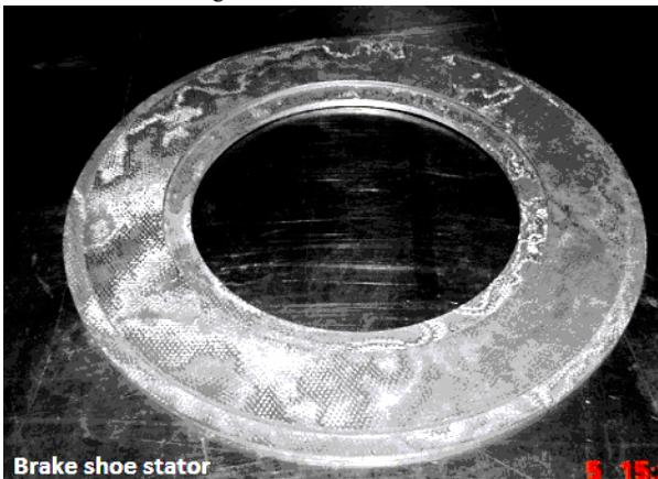
Figure 5 Carbon/Carbon stator
