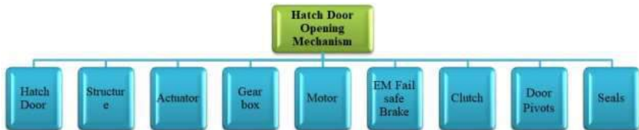
Figure 5.22 Hatch Door Opening Mechanism- Major Subsystems
