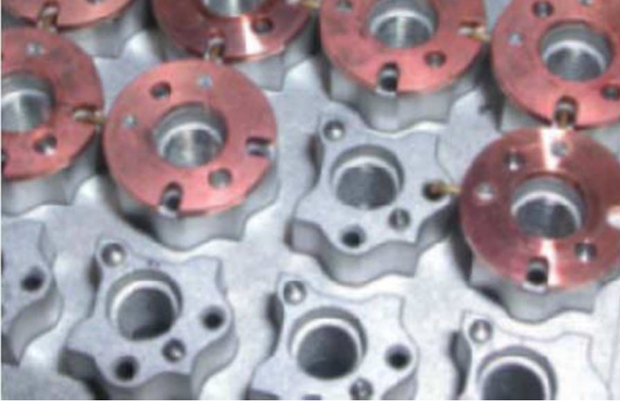
Fig. 3. Array ground plane and bricks with feeding pins.
