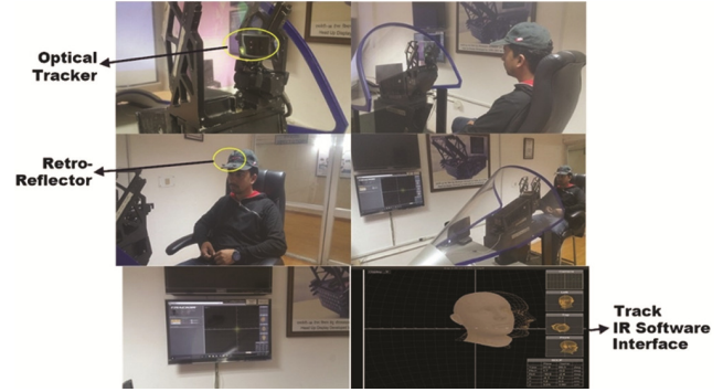
Fig.1 — Experimental Setup of Optical Tracking System with software interface
