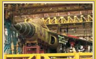
Main Airframe Static Test Rig
