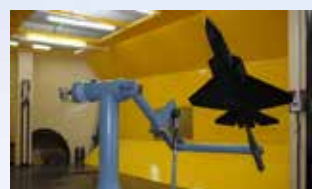
AMCA Model in Forced Oscillation Rig
