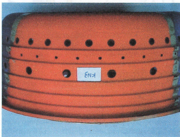
Fig.23 Thermal painted combustor liner (before paint test) and full-field temperature data revealing isothermal patterns
