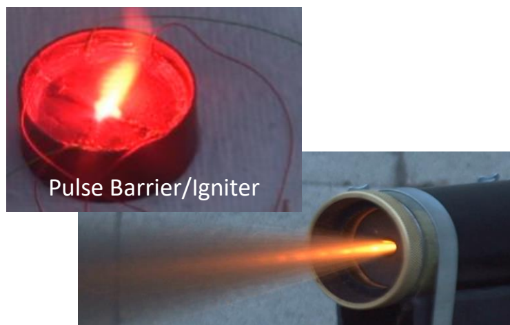
Figure 8 Phoenix™ ePropellant Barrier-Igniter Motor Demonstration
