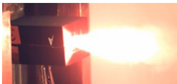
Figure 4, Phoenix ePropellant Small Thruster 5
