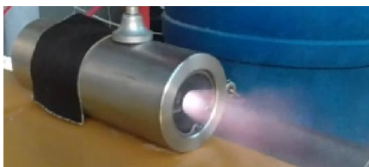
Figure 1, Small Electrically Activated Solid Propellant Thruster 5
