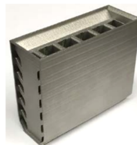
(e) M2HX, fabricated using Inconel 718 31
